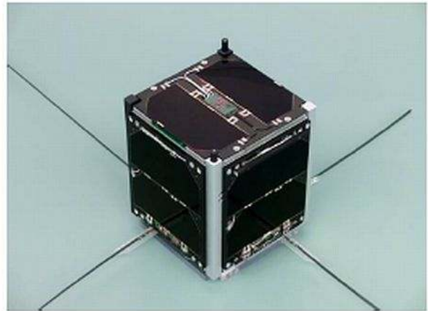
The actual FUNCube-1 spacecraft after an antenna deployment test
